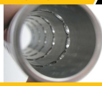
When deburring cross drilled holes using the Flex-Hone, it is helpful to first stroke and rotate the tool in a clockwise direction and then remove the tool from the bore, reverse the spindle and then stroke and rotate in a counterclockwise direction. This promotes a more symmetrical deburring pattern and prevents the burr from folding back into the cross-hole.
