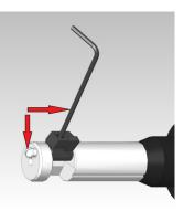
Apply a small amount of serviceable Loctite provided to thread of screw. Hand tighten set screw, being careful not to overtighten. If second follow-up screw is provided, install and hand tighten.
