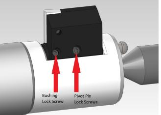
Using a hex wrench or something similar, rotate the Eccentric Bushing until required cutting radius is met. Re-tighten the set screw that is closest to the shank of the Autofacer to lock the Eccentric Bushing into place. Then re-tighten the Pivot Pin lock screws located midway between the width of the blade.
