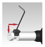
Apply a small amount of serviceable Loctite provided to thread of screw. Hand tighten set screw, being careful not to overtighten. If second follow-up screw is provided, install and hand tighten.
