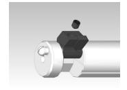
**TIP:** To verify that set screw is located on flat of Pivot Pin, loosen set screw slightly and attempt to pull Pivot Pin out of tool. The pin should only be able to slide until the set screw gets caught on the end of the Pivot Pin flat.
